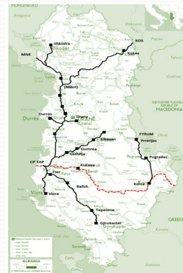
Existing and proposed gas transmission networks
