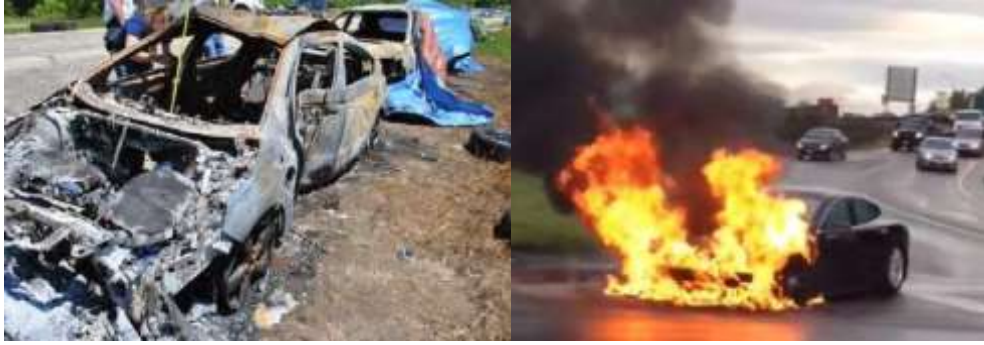
Figure 80 results of electrical fire caused by batter malfunction on EVs - Chevrolet Volt (left), Tesla model S (right) (source: S Kjosevski et al.)
