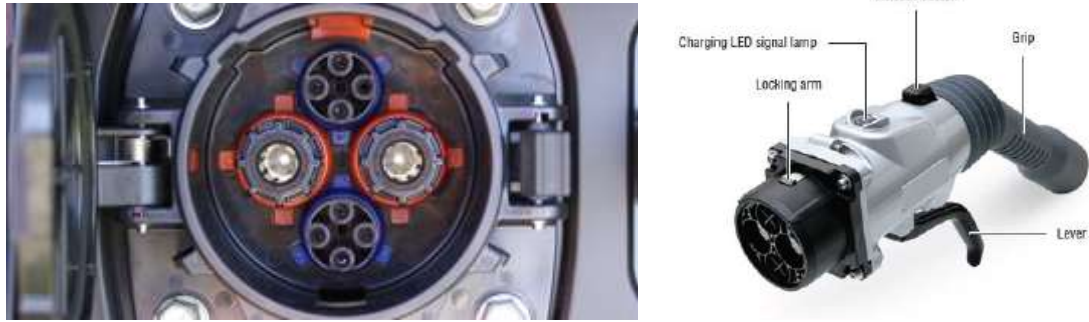
Figure 75 CHAdeMO plug and socket.
