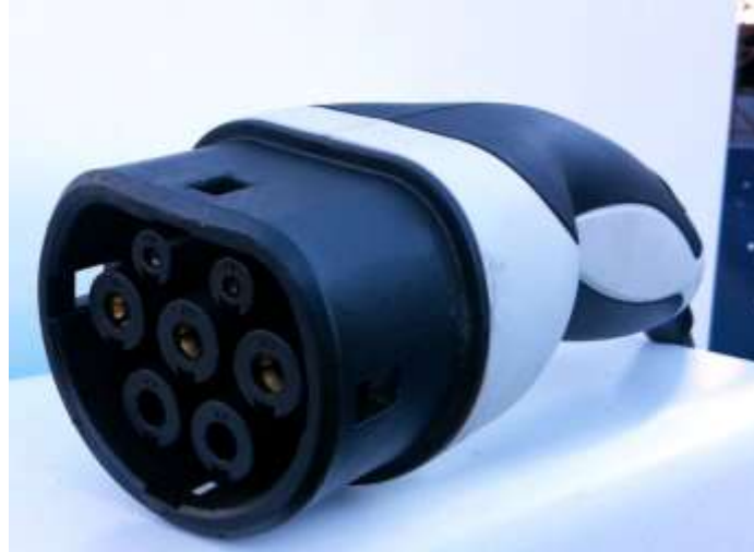
Figure 73 Type 2 coupler, Mennekes (source Hadhuey)
